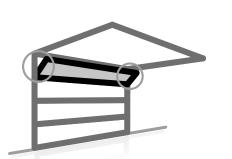
Garage ventilation feature is enabled by tilting the top panel without the need to lift the door. The bottom panel remains seated against the floor.
