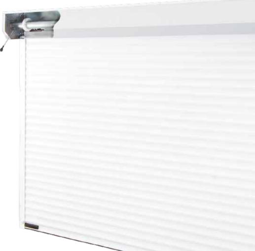
Gliderol Insulated Roller Doors take up very little space inside your garage. The standard configuration, using 77mm foam filled lath, requires 300mm of headroom and is supplied with 70 or 90mm guides depending on specification. The compact version, using 55mm foam filled lath, requires only 205mm of headroom and is supplied with 65mm guides.
